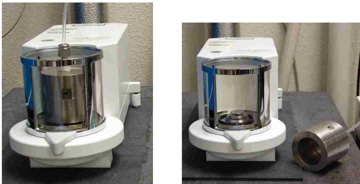
Figure 10-1. The Metler UMX-2 ultramicrobalance has a resolution of 100 ng and is used to directly measure the mass of analyte absorbed into the polymer film. The flowcell is a capped stainless steel cylinder, which envelopes the weigh-pan assembly.
