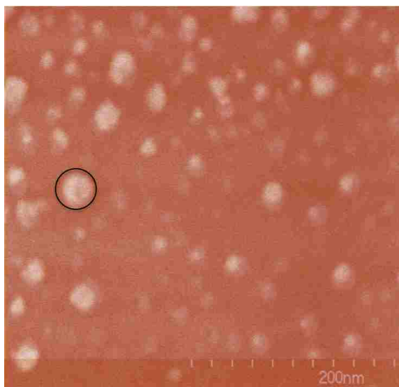
Figure 5.7: Binary image of Figure 5.6 showing that the particle that grew after vacuum ageing has no faint halo around the particle, like most particles that have decreased in size from evaporation
