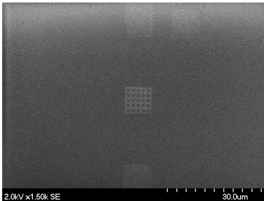
Figure 3.4: The entire FIB grid in a low magnification SEM micrograph that includes the lines that guide to the FIB grid, which can be seen at the top and bottom center of the micrograph.
