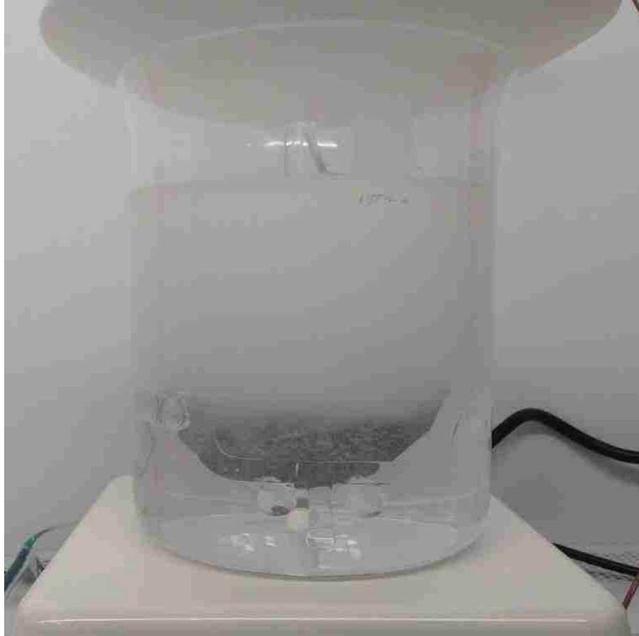
Figure 3.1. A photograph of a 4-inch c-Si wafer on a quartz sample holder in the middle of thinning. The vigorously formed hydrogen bubbles mix the solution effectively at 90 °C in 50 wt.% KOH solution.
