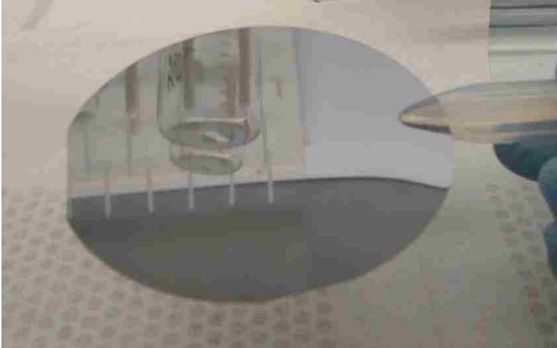
Figure 3.3. A free-standing 50- \mu\text{m} -thick 4-inch c-Si wafer. The thinned c-Si wafers can be handled by tweezers without being bent or broken.
