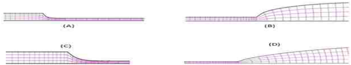
Fig 6. Various mesh layouts at different web speeds and pressures. (A) U_{web} = 7 \text{ cm/s} , P = -8.10E+5 \text{ dyne/cm}^2 ; (B) U_{web} = 7 \text{ cm/s} , P = 1.90E+7 \text{ dyne/cm}^2 ; (C) U_{web} = 0.1 \text{ cm/s} , P = -1.97E+4 \text{dyne/cm}^2 (D) U_{web} = 0.1 \text{ cm/s} , P = 8.70E+5 \text{ dyne/cm}^2
