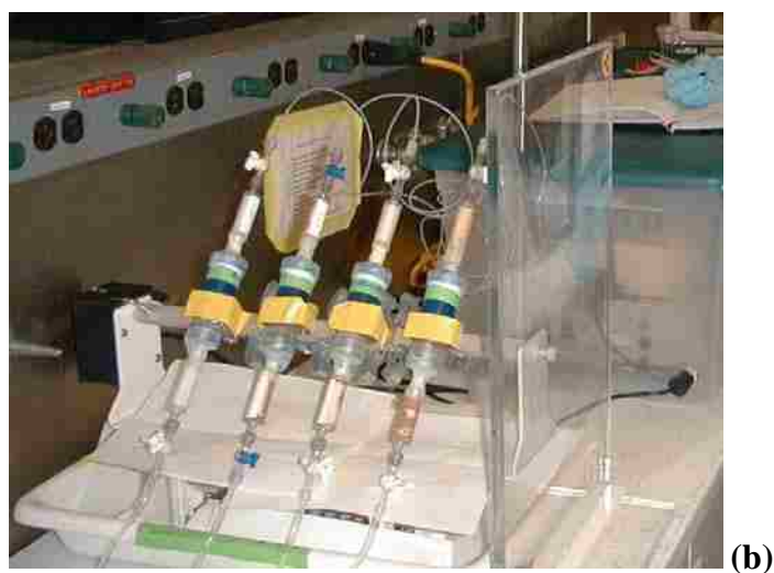
Figure 2.3. Schematic (a) and photo (b) of batch sorption reactor/flow desorption CSTR. The volcanic tuff is pre-sorbed with uranium and neptunium (separately) prior to the column flow desorption. The column is placed on an end-over-end shaker to maximize tuff-solution contact during both the sorption and desorption phases.
