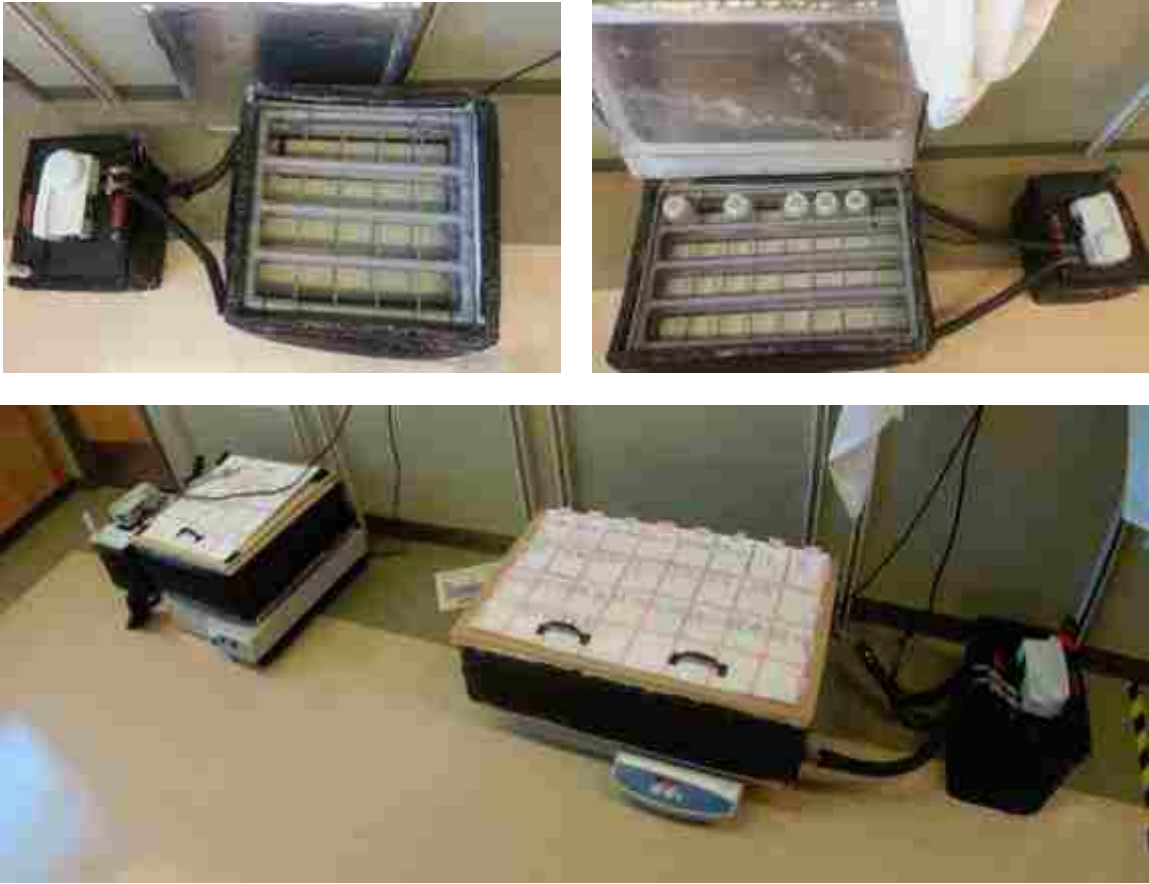
Figure 24: Bench Scale Controlled Temperature Baths; Unit 1: 20 sample capacity (top left), Unit 2: 32 sample capacity (top right); Heat baths on shaker tables (bottom)
