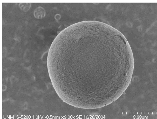
Figure 7.5: SEM micrograph of the nucleosil particle after base/peroxide wash
