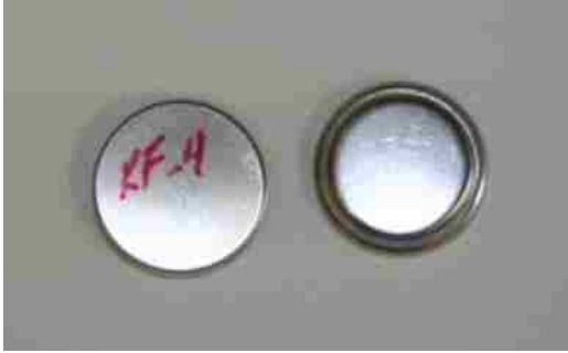
Figure 31 – Complete 2032 coin cell assembly containing robocast cathode.
