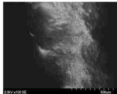
Figure 48 – SEM image of the printed polypropylene film at 2.0 kV.
