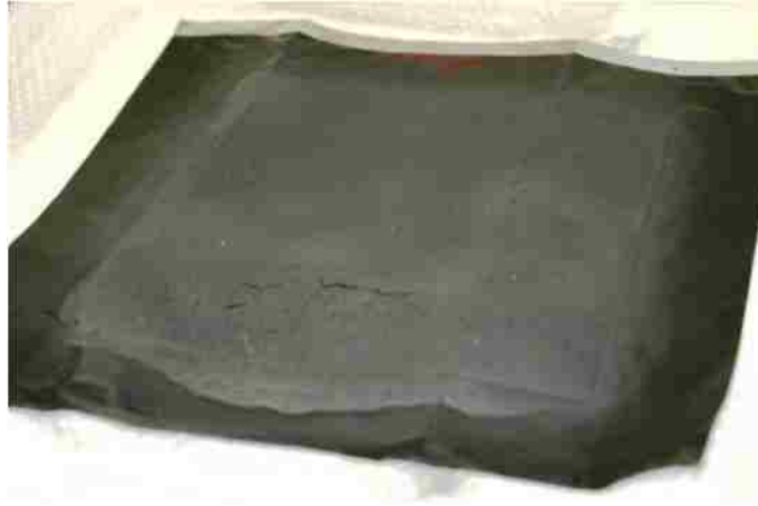
Figure 29 – Example of electrode made using pneumatic atomization on the robocasting machine. The substrate used for deposition is carbon coated aluminum.
