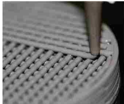
Figure 14 - Robocasting example of a part being casted using the extrusion technique.
