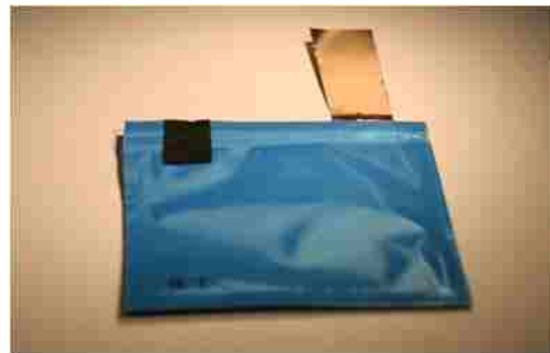
Figure 40 – Pouch cell constructed for evaluation of robocast battery cathodes for pulsed power application.
