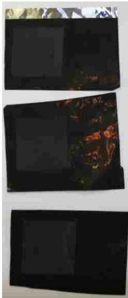
Figure 30 – Robocast cathodes as prepared.
