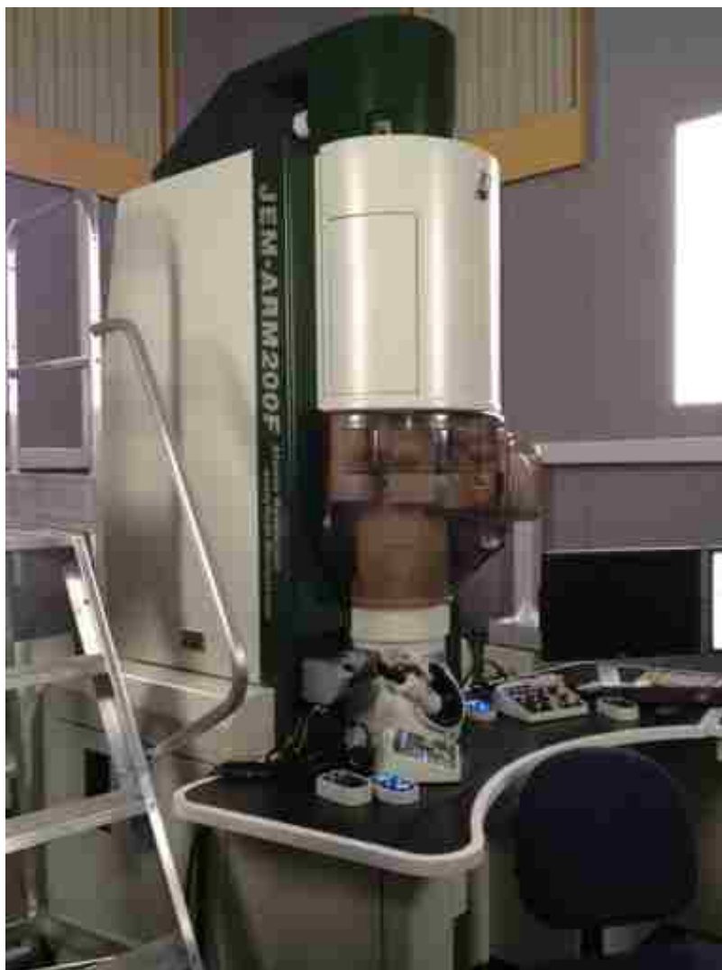
Figure 3.6 Image of aberration corrected JEM ARM 200F (ASU)
