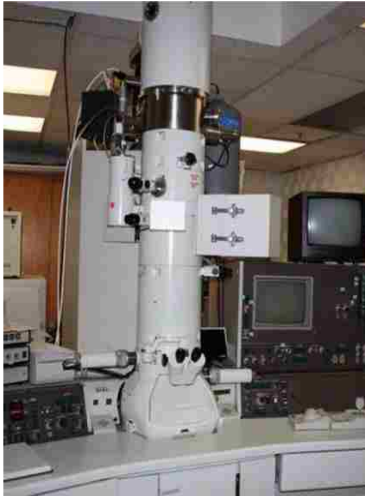
Figure 3.5 Image of JEOL 2010F STEM at the University of New Mexico
