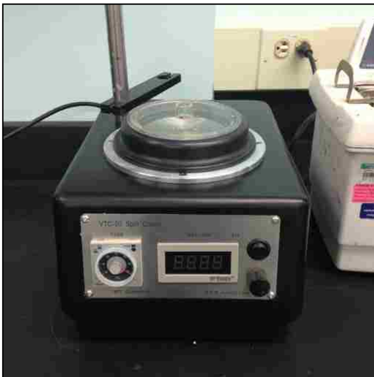
Figure 4.1 TC100 AG Desktop Spin Coater used for spin coating samples
