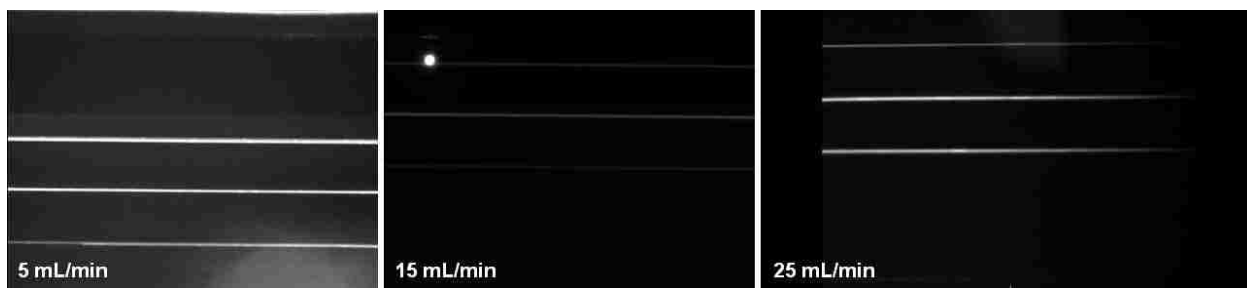
Fig.7.3 10.2 \mu m Nile Red polystyrene particles focused into 3 nodes in one of the channels in the microfabricated 100-channel flow cell at 5,15 and 25 mL/min flow rates
