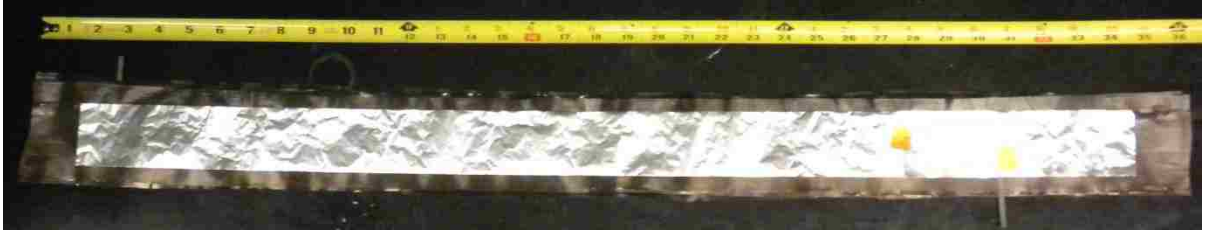
Figure 19. 3 ft capacitor (prior to rolling) of extruded 10% (w/w) trioctyl trimellitate in S-POW.
