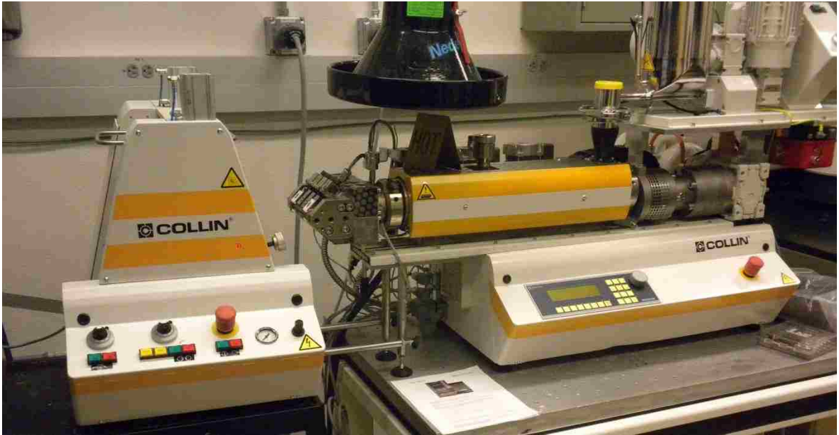
Figure 16. Dr. Collin® extruder used for in-house extrusion of S-POW.
