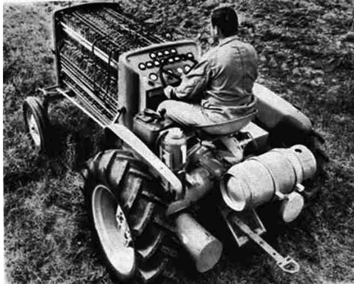
Figure 1-3. Alkaline fuel cell tractor developed by Allis-Chalmers Manufacturing Co.
