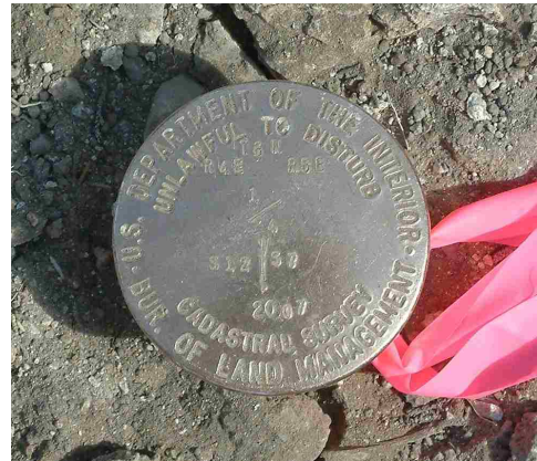
Figure 36. Close up showing the new corner brass cap’s markings.
