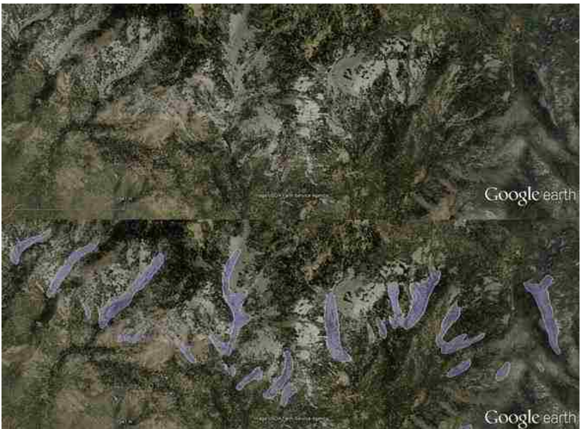
Figure 3.11 Rock glacier digitization in the Capitan Mountains. At least 26 rock glaciers are visible in the top image. Many rock glaciers meet and flow over other rock glacier structures; thus only 21 polygons were created as seen in the bottom image. Source: Adapted from Google, NAIP 2012
