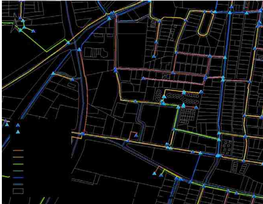
Figure 3.10. Parcels, streets, and the water system, represented by junctions with demand, junctions without demand, and pipelines, are shown.
