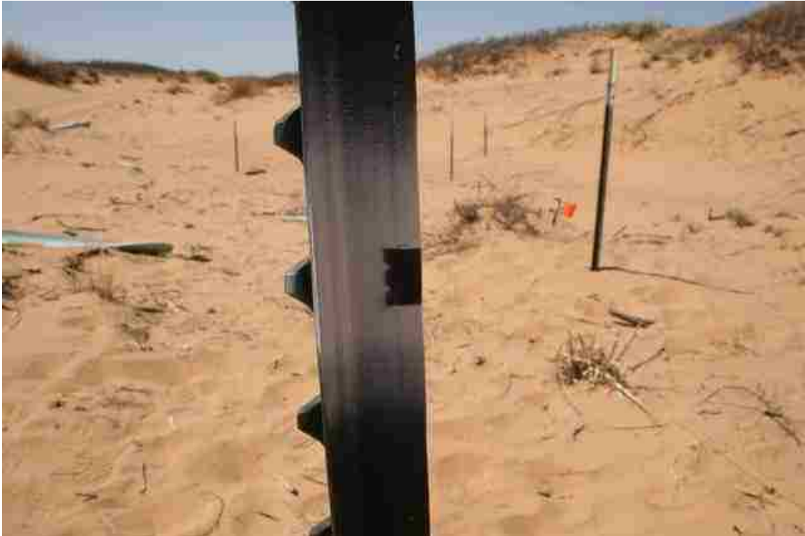
Figure 13: Spray paint showing where the binder clip will be placed each time the leveling thread needs to be attached for measurement. Photo: Knutt Peterson
