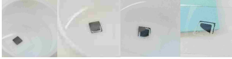
Figure 4.13: p -type InAsSb VDP processed sample in the HF-based solution. The HF-based solution will etch away the GaSb substrate, the AlAsSb etch-stop, the GaSb buffer layers, and begin to etch the InAsSb epilayer since no photoresist sidewall protection was used.
