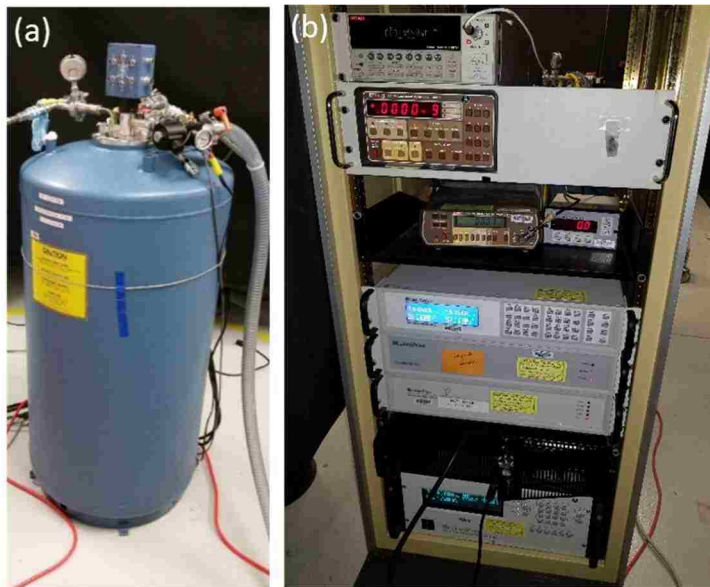
Figure 3.4: LakeShore Cryotronics Hall Measurement System, (a) Model 9509 cryogenic dewar with sample insert mounted in the dewar, (b) electronics equipment rack.
