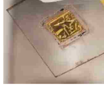
Figure 6.13: Sample “wrinkles” during an attempt to perform photolithography after substrate removal to fabricate top contacts. The sample is shown as it looks through the sapphire carrier (substrate side down).
