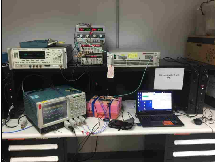
Figure 48: MCU Upset experiment setup.
