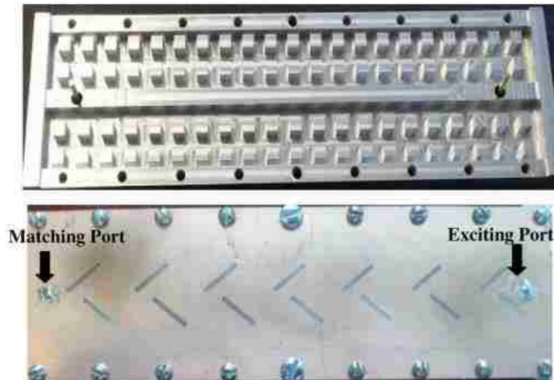
Figure II.1: (a) The configuration of the dipole layer on top of the slot, (b) fabricated prototype of the parasitic dipoles on top of a slotted waveguide array.[29]
