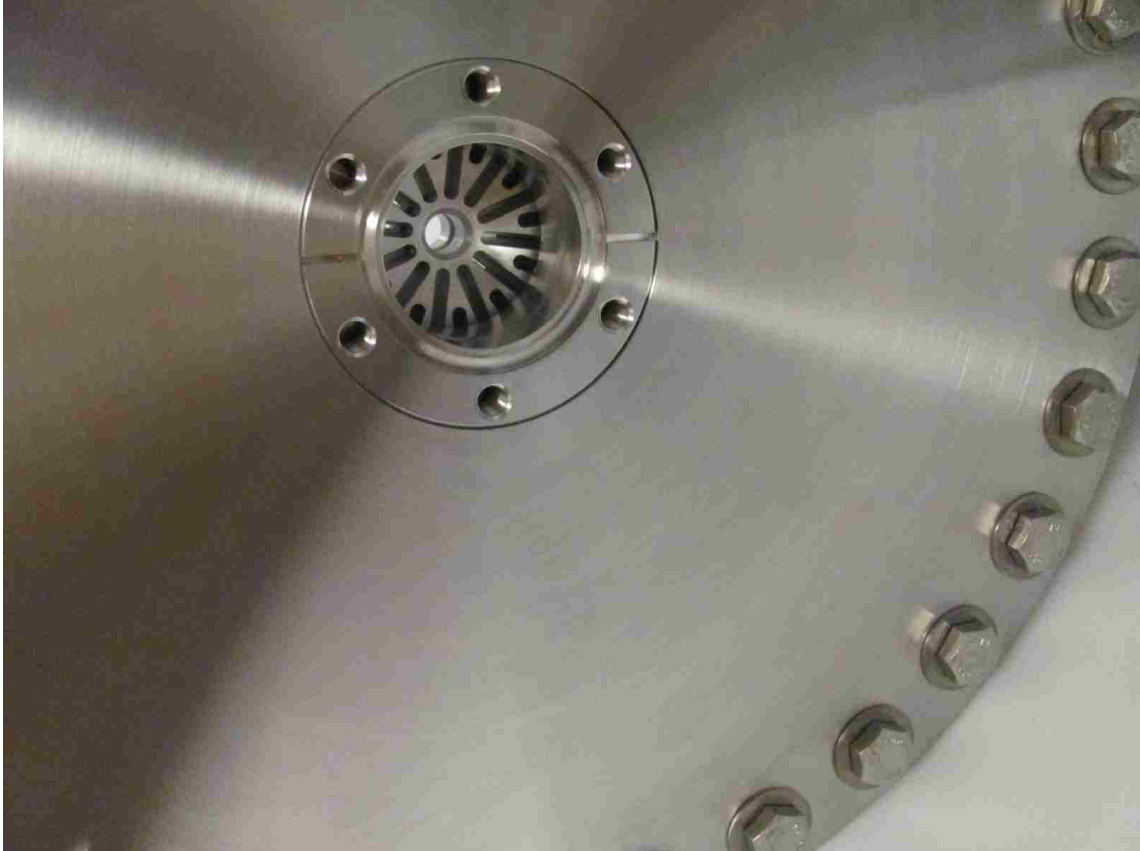
Figure 1.1.6: The cavity of Figure 1.1.5 sandwiched between two 12" to 2 \frac{3}{4} " flange reducers to make it compatible with Jlab's Injector Test Facility beamline.
