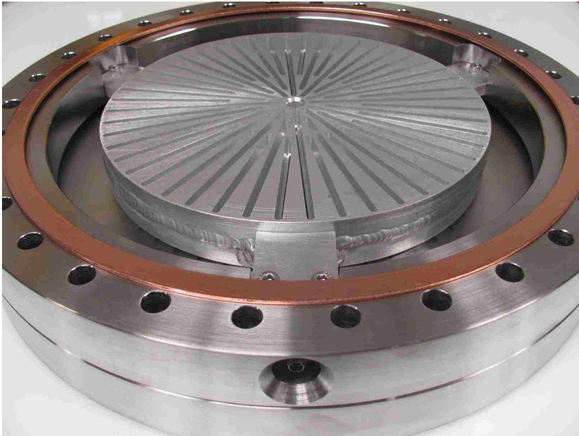
Figure 1.1.5: A beamline compatible harmonic cavity constructed for testing on the Jlab Injector Test Facility.
