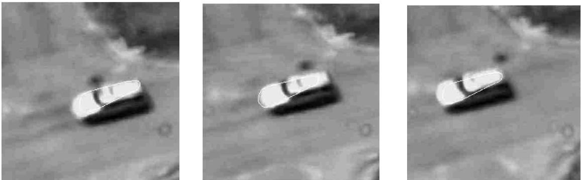
Figure 4.11 Van through the intersection, frames 1, 9, and 16 with convex shell applied
