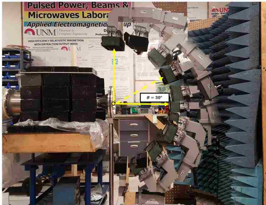
Figure 3.13 Vertical field sweep with waveguide positioned at every 15 for a full 180 degrees (Dmitrii Andreev provided photograph).
