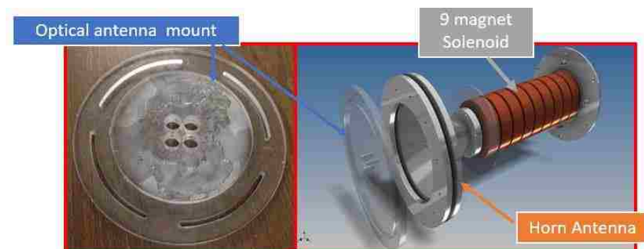
Figure 3.25 Optical mount for the collimating lenses that attaches to the front of the antenna.
