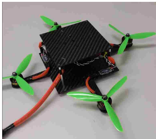
Figure 2.5: LoboDrone v1.0 quadrotor frame with actuators.
