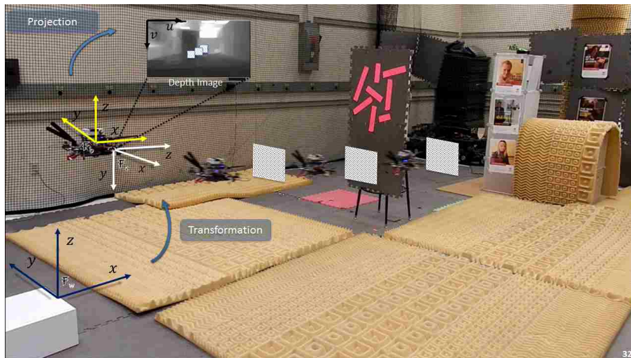
Figure 3.4: Computation of the artificial shields and their transformations and projections in the depth image space.
