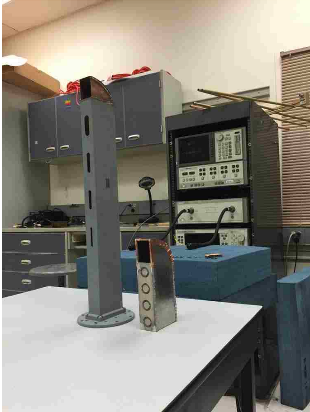
Figure 5.1: S-band narrow-wall complementary-split-ring slotted waveguide antenna aligned with the S-band narrow-wall longitudinal slotted waveguide antenna.
