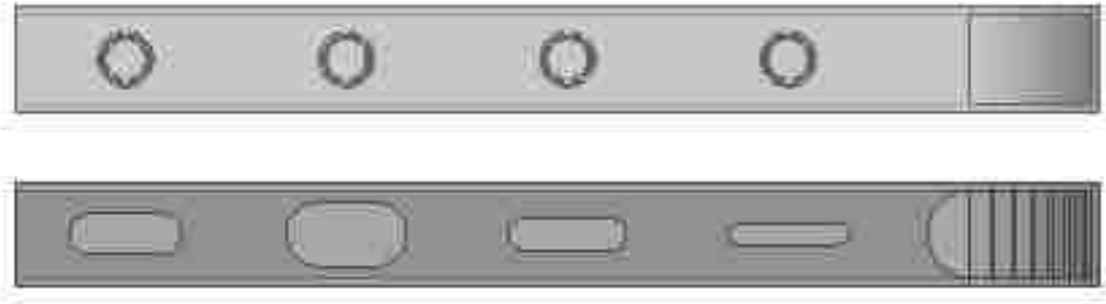
Figure 3.3: Comparison of the CSR-SWA with the longitudinal slot array (same inter-element spacing)
