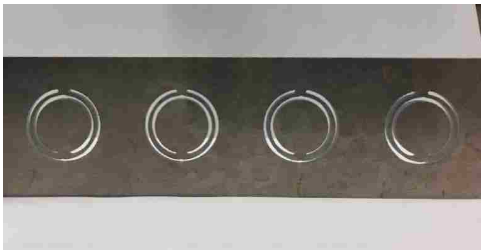
(b) Complementary-split-ring slots cut by Waterjet Cut Inc.
