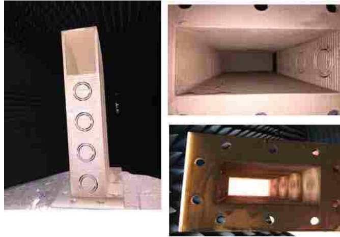
Figure 5.14: A 3D printed CSR-SWA applied with MG chemical 843 conductive coating.
