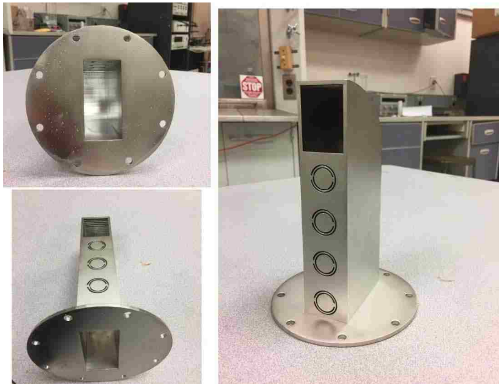
Figure 5.19: Bluestone printed CSR-SWA plated with copper by RepliForm Inc.
