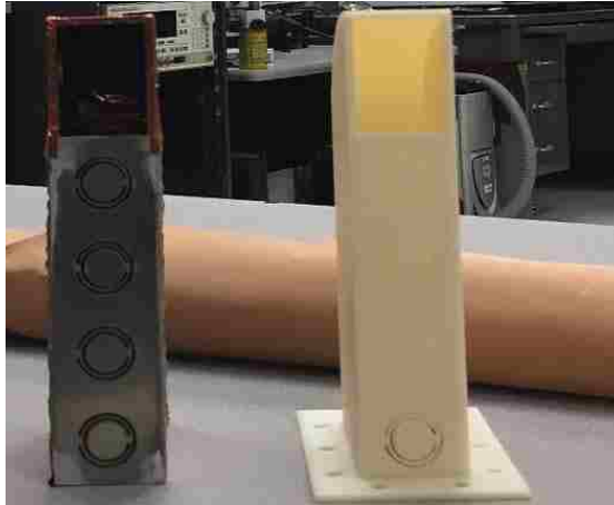
Figure 5.12: 3D printed CSR-SWA (on the right) and aluminum CSR-SWA. Antenna one the left is the metallic version.
