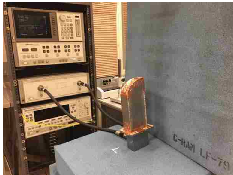
Figure 5.5: S parameter measurement set-up for the S-band narrow-wall complementary-split-ring slotted waveguide antenna.
