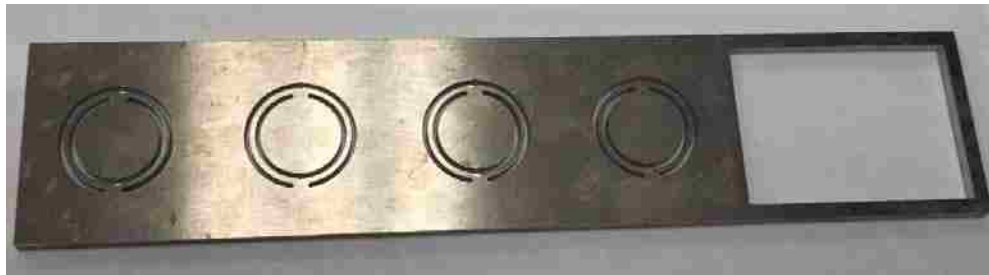
(a) aluminum plate as one the narrow-wall of the waveguide
