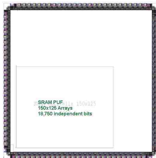
Figure 10: Floorplan and placement of the SRAM PUF.
