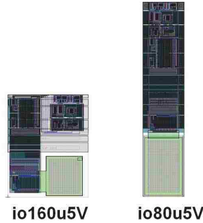
Figure 2: Two types of pad libraries: io160u5V with 160µm pitch and io80u5V with 80µm pitch.
