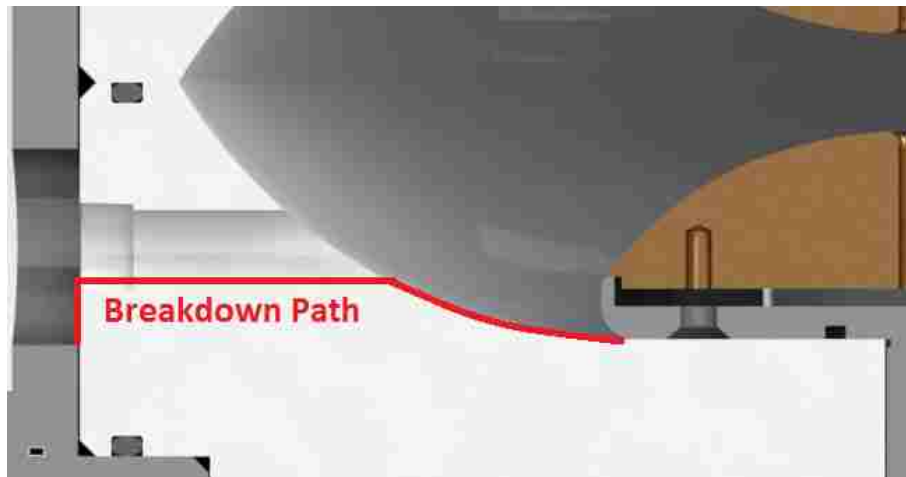
Figure 5.1: Surface breakdown path shown along the Rexolite ® insulator in red.
