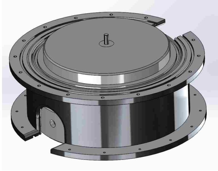
Figure 5.3: Rendering of the switch housing with a modified clearance around the pressure fitting.
