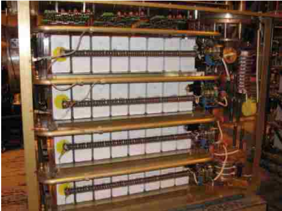
Figure 2.2: PFN Marx generator used to drive the DARHT Axis-II induction cells [9].
