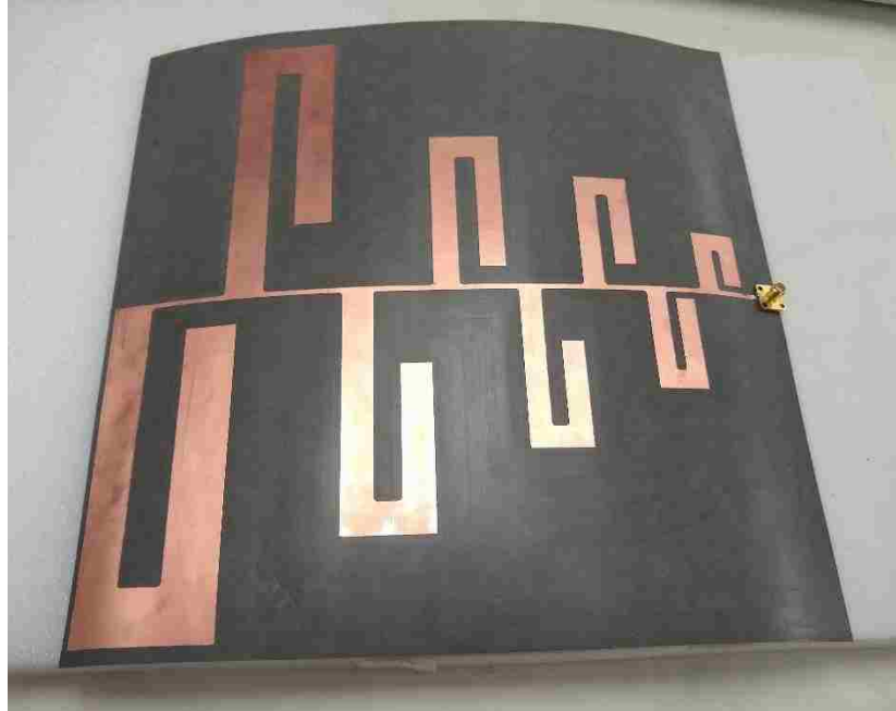
Figure 41 - Fabricated LPDA for bandwidth 300 -1000 MHz
