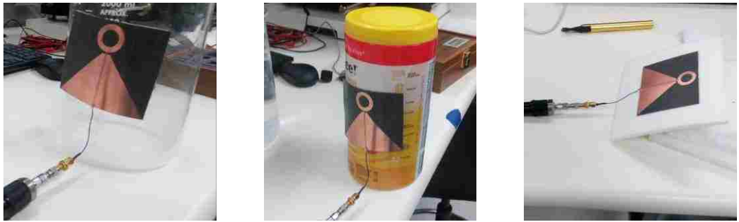
Figure 26- The annular monopole when stuck on multiple surfaces
