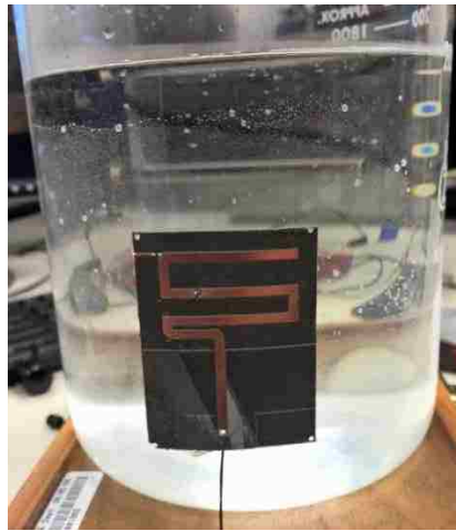
Figure 34 - The meandered monopole stuck on the surface of a beaker filled with water.
