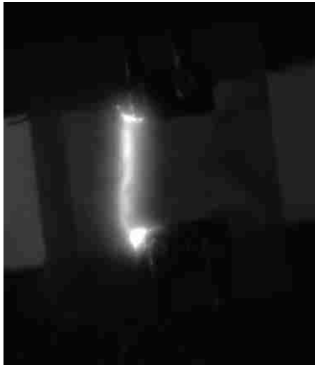
Figure 52: Hextech AlN filament at 1481V, 13mJ laser pulse
