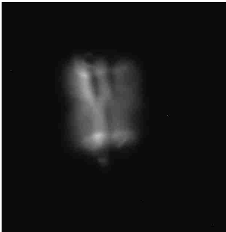
Figure 49: AMMONO GaN filaments at 1247V, 2.7mJ laser pulse, 1500pF input capacitor, 2x attenuator
