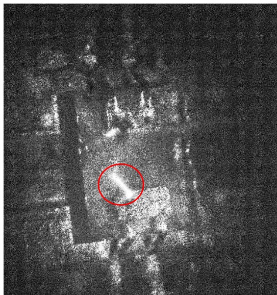
Figure 21: Kyma Lot 1 filament at 976V, 2mJ laser pulse. Filament circled in red
