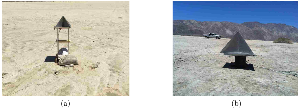
Figure 4.3: Targets without no concealed vibrating sources. (a) Rocking quad-corner reflector; (b) sliding quad-corner reflector [31].
