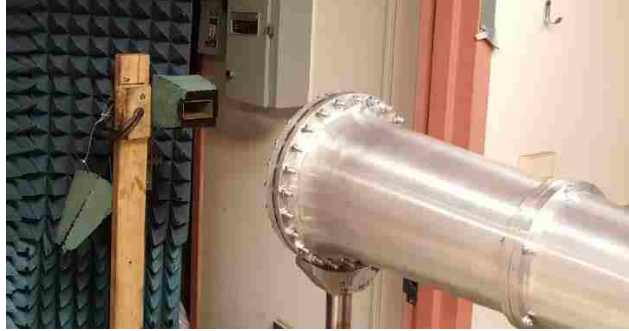
Figure 4-12: Photograph of the rectangular waveguide sensor in front of the cylindrical horn antenna.
