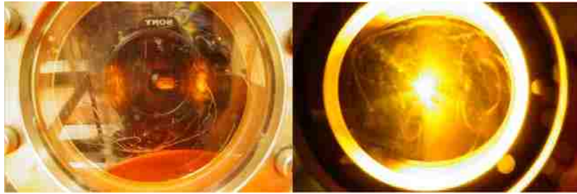
Figure 4-3: Photograph of the oil gap switch pre-fire (left) and during operation (right).
