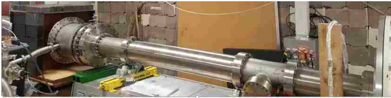
Figure 4-8: Photograph of the final assembly of the permanent magnet onto the PULSERAD accelerator.
