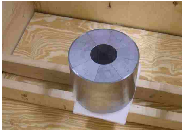
Figure 4-4: Photograph of the NdFeB permanent magnet as-delivered at UNM.
