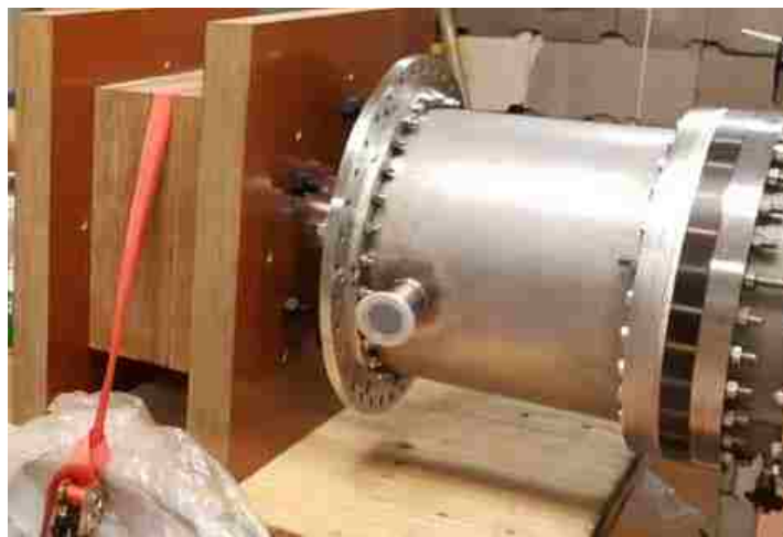
Figure 4-6: Photograph of the permanent magnet installed in a phenolic housing.
