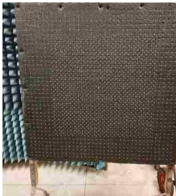
Figure 4-13: Photograph of the neon bulb array used for mode characterization.
