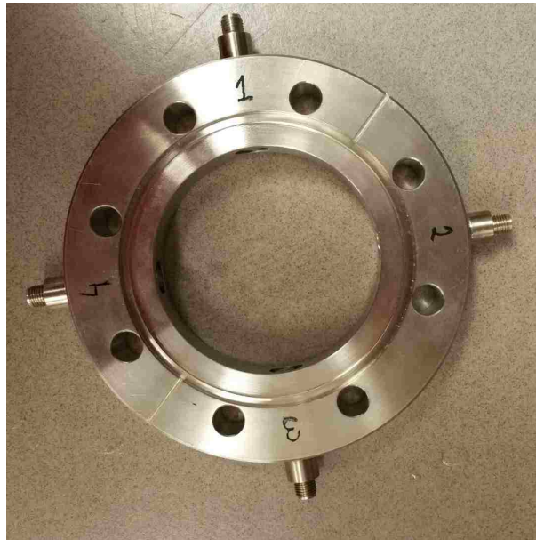
Figure 1.2: The Beam Position Monitor flange, SMA connectors for each pick up are shown at the numbered positions.
