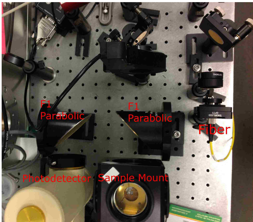
Figure 3.2: Basic setup of photoluminescence-based measurements, consisting of two F1 parabolic mirrors to collimate and focus the emission of the sample under test.
