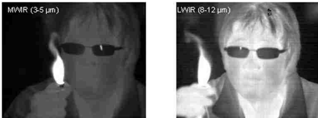
Figure 2.2: Two pictures that have taken using the same DWELL infrared FPA. While the bias of the detectors are uniform across the FPA, in each picture, the bias voltage is selected to optimize the responsivity at MWIR in the left or LWIR on the right [36].
