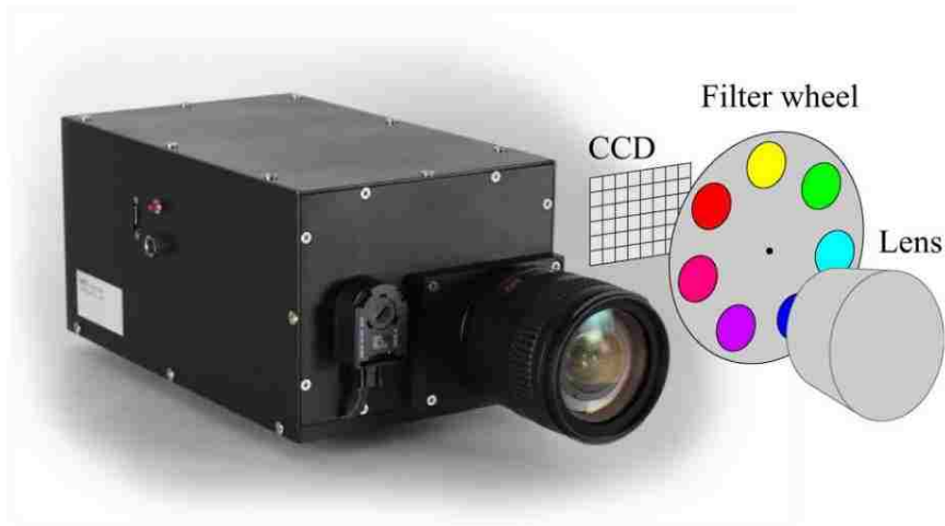
Figure 2.1: A multispectral camera that employs seven bandpass filters to separate different bands on the left and an iconic representation of the internal block diagram on the right [33]
