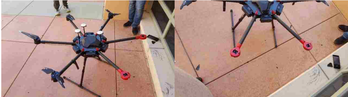
Figure 4-10. Damage to the UAS propellers and front motors from UNM crash.
