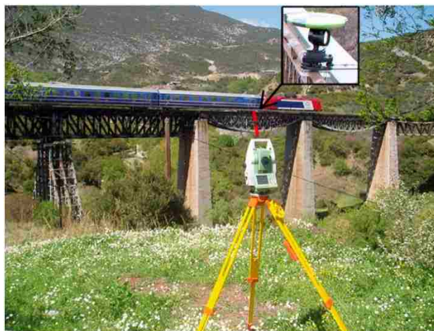
Figure 2-5. Railway bridge monitoring using a robotic total station (Psimoulis and Stiros, 2013)
