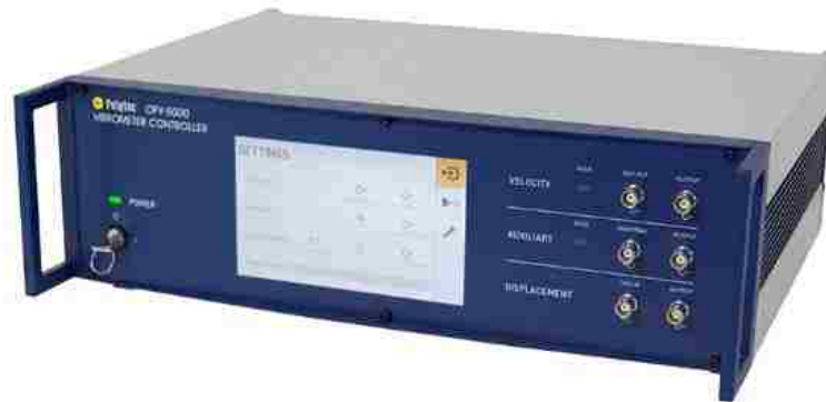
Figure 3-2. OFV-5000 Touch - Vibrometer Controller (Polytec 2017)
