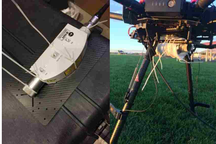
Figure 4-17. Vibrometer assembly to the UAS.
