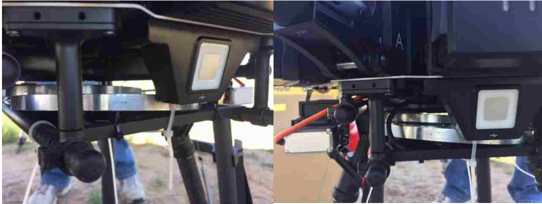
Figure 4-9. UAS attached with dead weight for test flight
