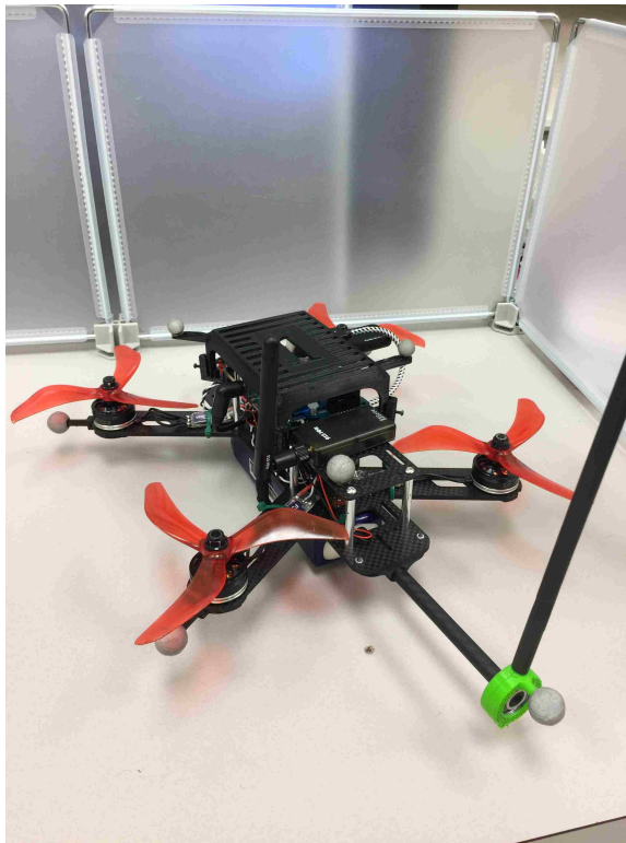
Figure 5.9: Quadcopter with attached pendulum. Custom designed and printed parts to cover Odroid XU4, hold markers, attach the pendulum to quadrotor and attach pendulum to ball bearing.
