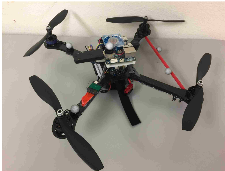
Figure 2.2: AscTec Hummingbird quadrotor with Odroid XU4 microprocessor on top of it and Vicon markers attached.
