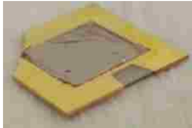
FIG. 3.28 DEMONSTRATION OF GASB AND CVD DIAMOND INTEGRATION BY BOTTOM-SIDE APPROACH AFTER STEP 3
