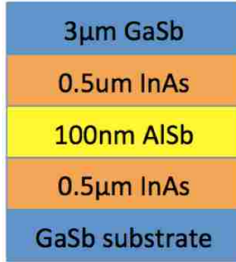
FIG. 2.17 SCHEMATIC OF ELO STRUCTURE FOR INAs/ALSb/GASb MATERIAL SYSTEMS
