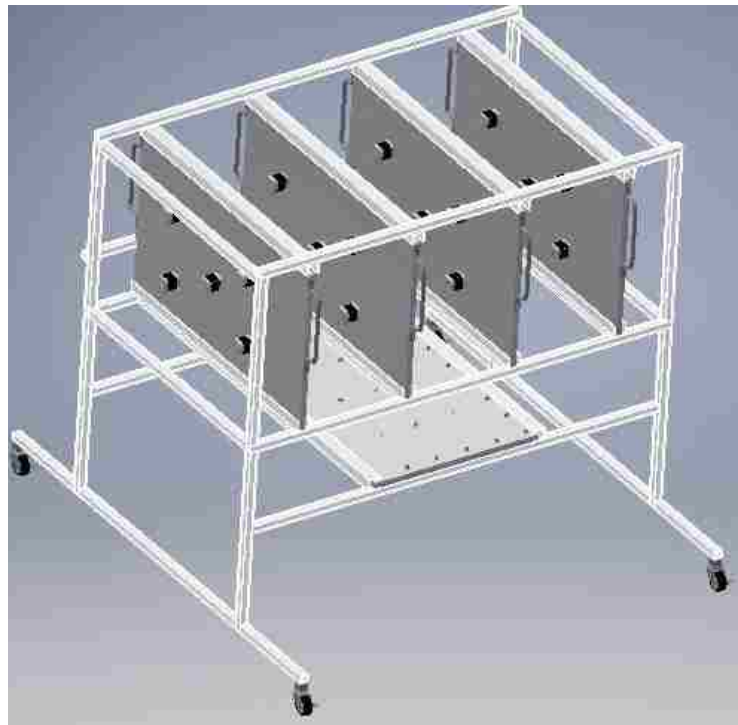
Fig. 3.1. CAD drawing of five quasi-2D ray chaotic cavities that will be interconnected in an arbitrary manner.
