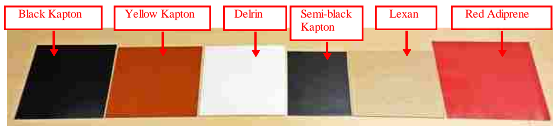
Figure 8: Dielectric samples tested.
