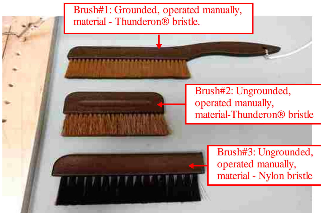
Figure 9: Brush tools for dielectric surface charge removal.
