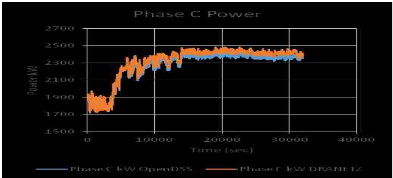
FIGURE 7 REAL POWER SIMULATION VALUES COMPARED TO THE METERING DATA GATHERED FROM THE FIELD.
