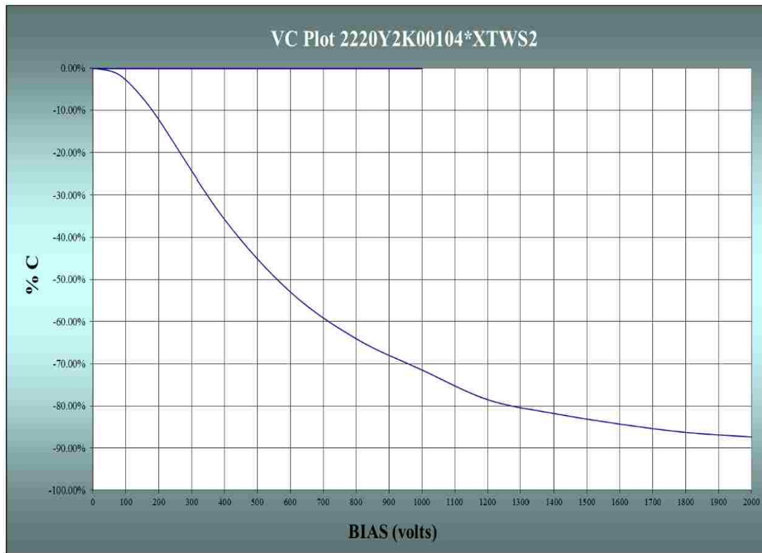
Figure 18: C-V plot for Knowles 2220Y2K00140*XTWS2
