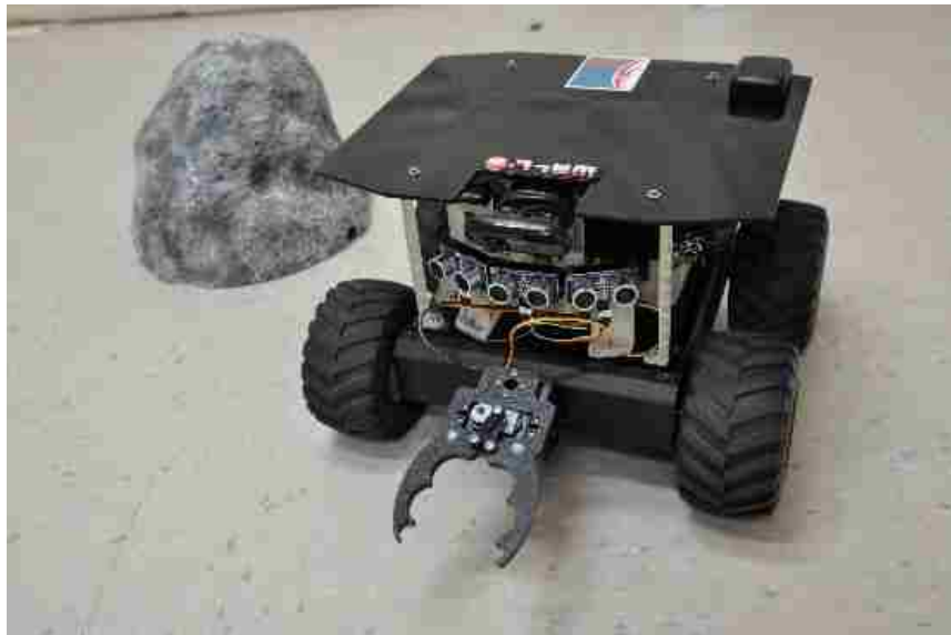
Figure 4.14: Swarmie With Gripper
