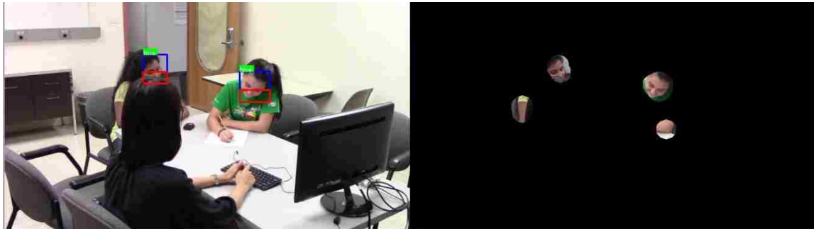
Figure 3.20: Correctly identified faces (left) and skin regions that were sent to KNN (right).
