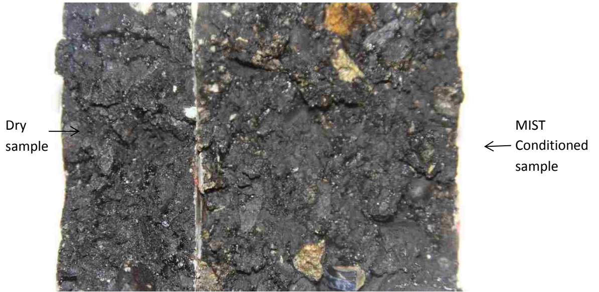
Figure 6.2 Photographic view of dry and MIST conditioned samples
