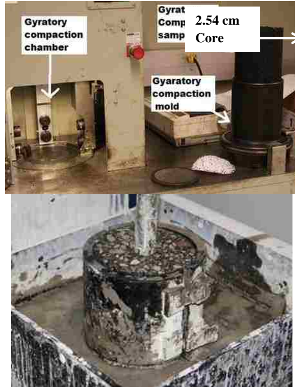
(a) Gyrotory Compactor (b) Coring of Sample
