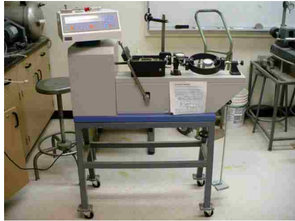
(b) Direct shear test setup
