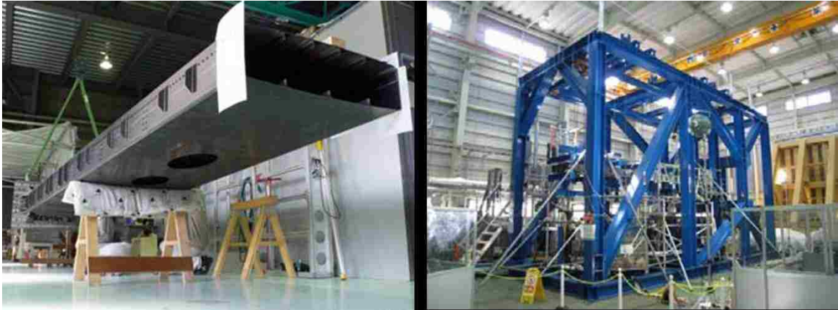
Figure 2-3: Composite Wing Box (Right) and Structural Testing Equipment Used by Murayama
