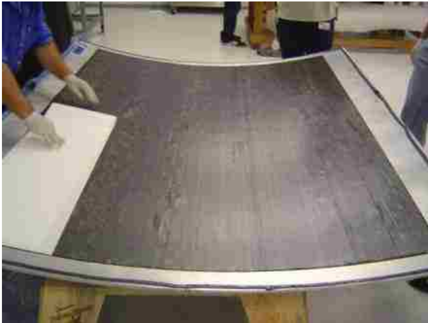
Figure 3-8: Carbon Pre-Preg Skin Plies Being Laid Up on Caul Plate
