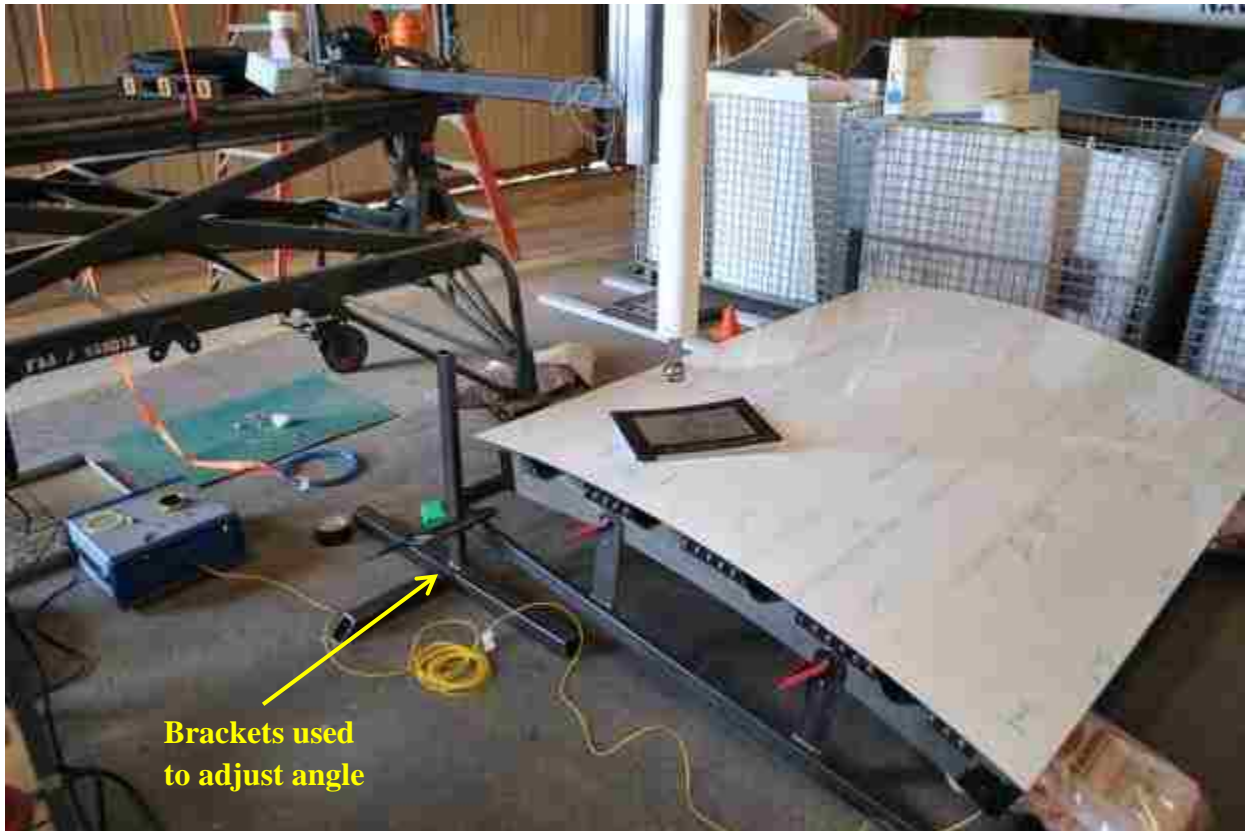
Figure 3-27: Panel A Set Up for Drop Weight Impact Testing
