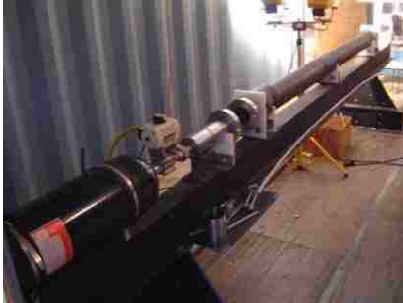
Figure 3-18: Gas Gun used for High Velocity Ice Ball Impacts Testing Showing the High Pressure Gas Tank, Pneumatic Actuator, Breach and Barrel
