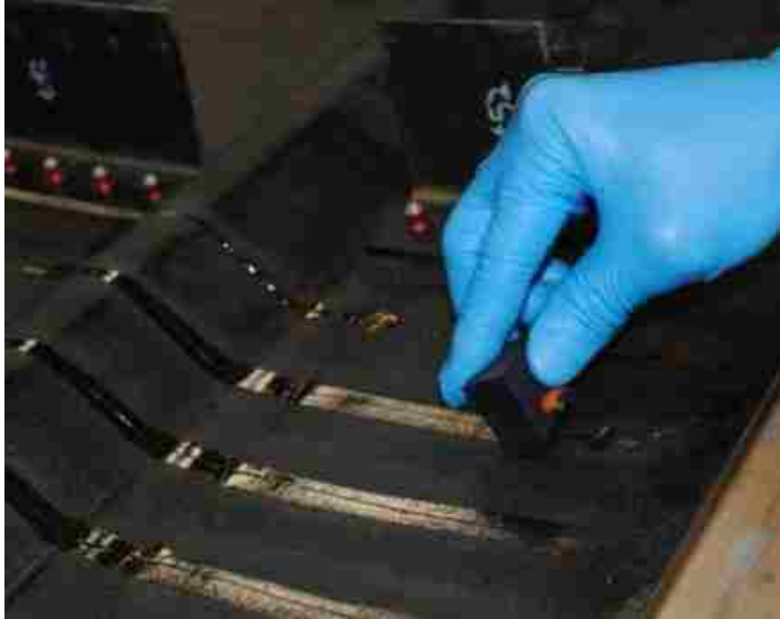
Figure 3-14: Thin Line of M-Bond GA-2 Adhesive Being Squeegeed Smooth Around Fiber Optic
