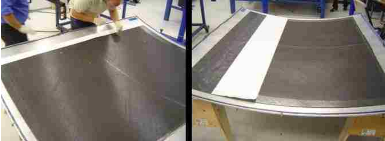
Figure 3-9: Fiber Optic Placed on Skin Layup and Subsequent Layer of Carbon Being Applied
