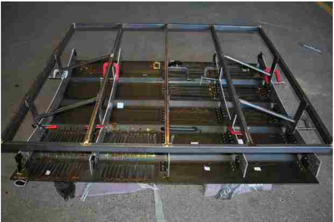
Figure 3-26: Panel A Clamped to the Steel Frame for Drop Weight Impact Testing
