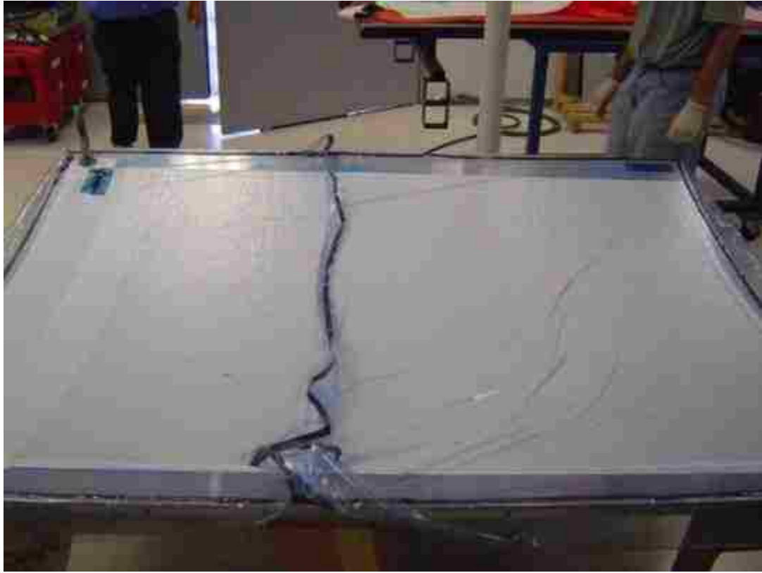
Figure 3-10: Skin Layup Bagged and Being Debulked
