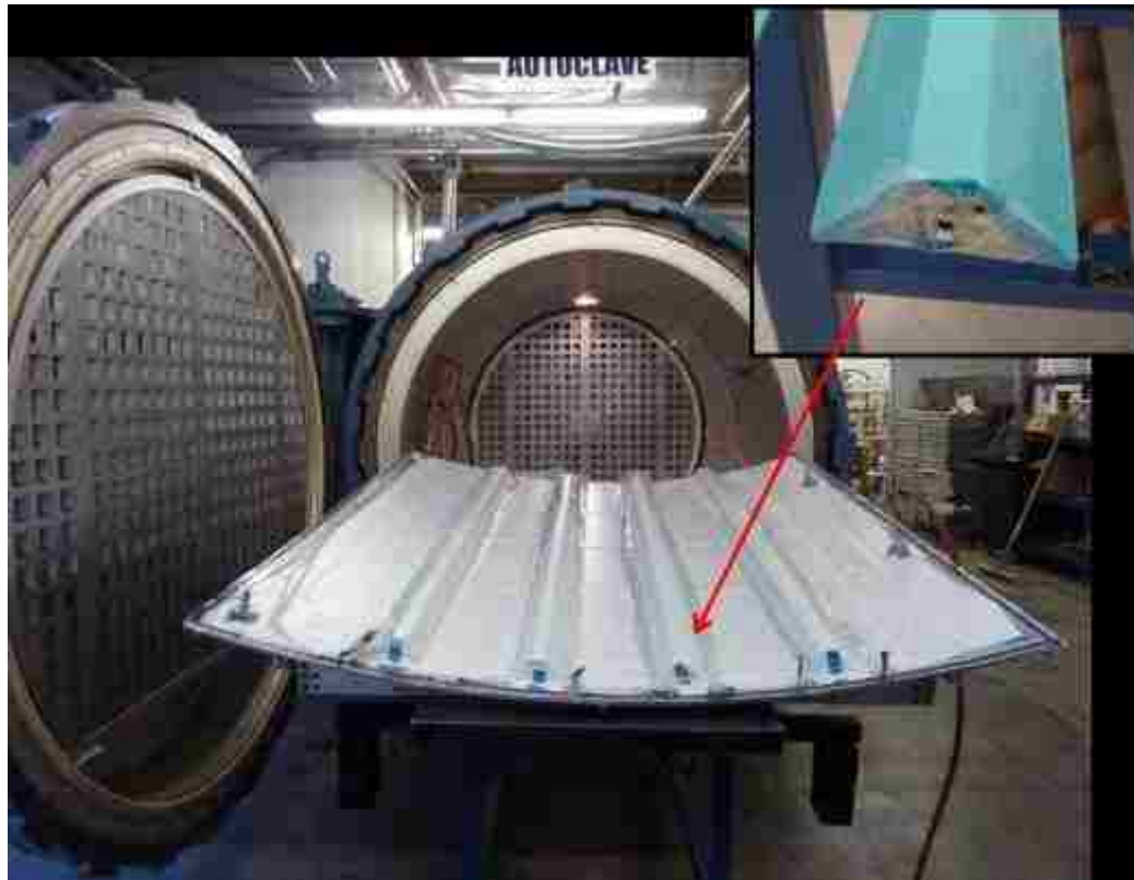
Figure 3-12: Autoclave and Silicone Stringer Molds used to Cure Panels
