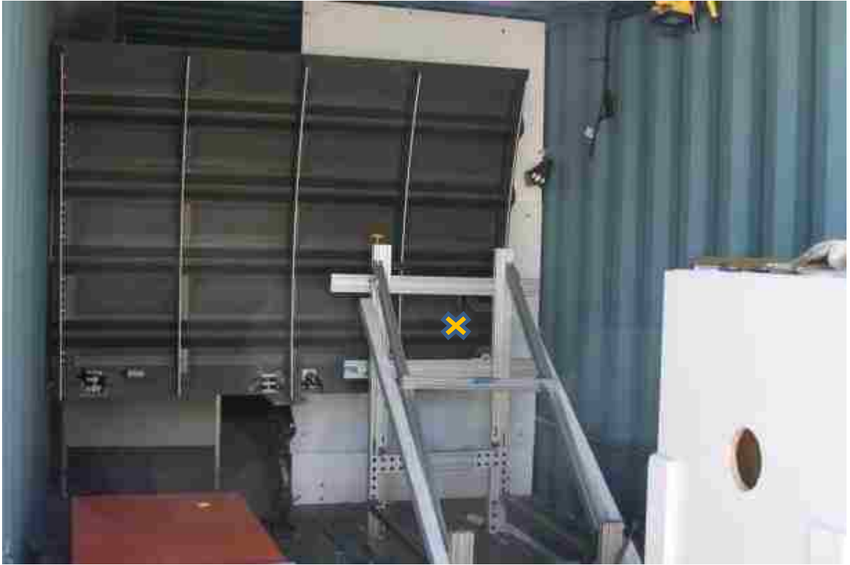
Figure 3-19: Panel Supported with Frame being Prepared for Impact Test
