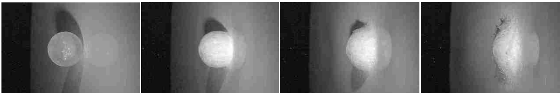
Figure 3-21: High Speed Image of Simulated Hail Impacting Fuselage Panel
