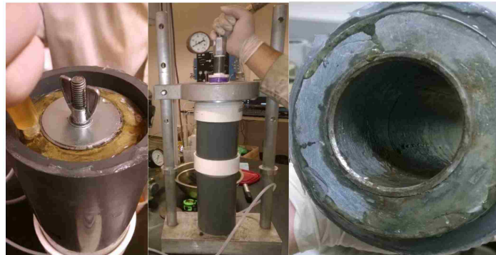
Figure 3.4: A flawed specimen is shown undergoing injection with an epoxy repair material (Stormont, 2014)
