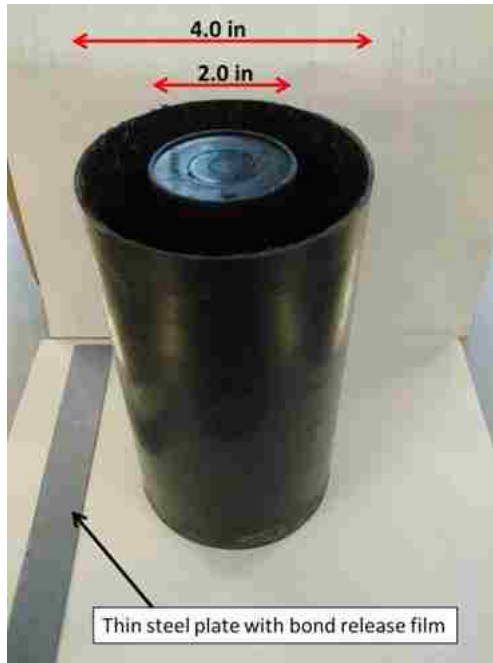
Figure 3.2: Laboratory wellbore mold of for lab-scale seal system
