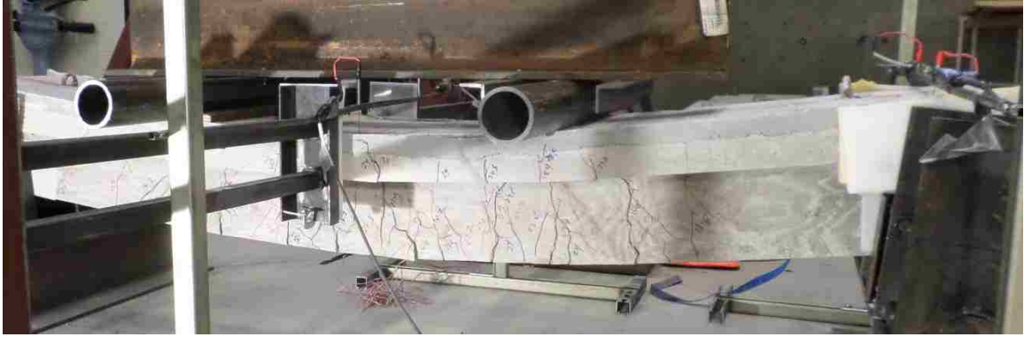
Figure 4.22: Cracks propagated in Beam-U
