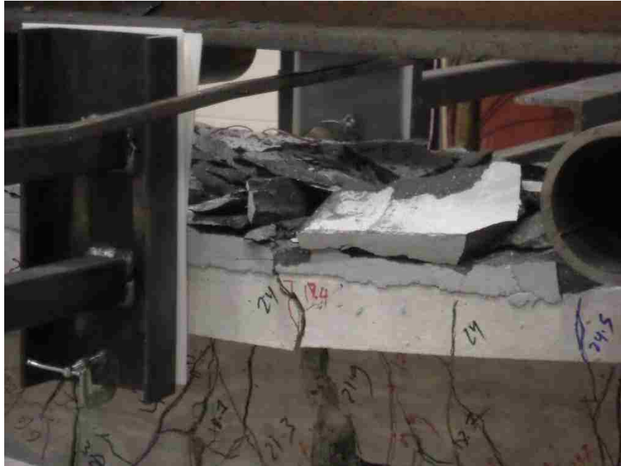
Figure 4.24: Crushing of UHPC top layer in Beam-U
