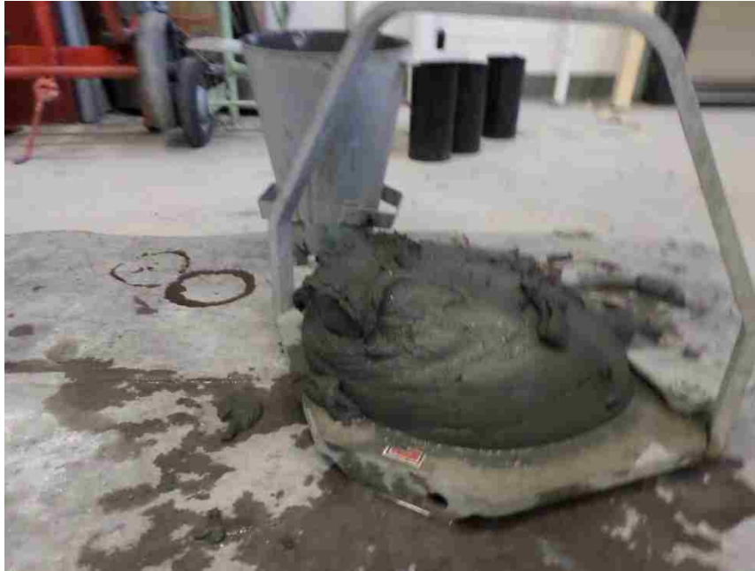
Figure 4.3 Slump of UHPC1
