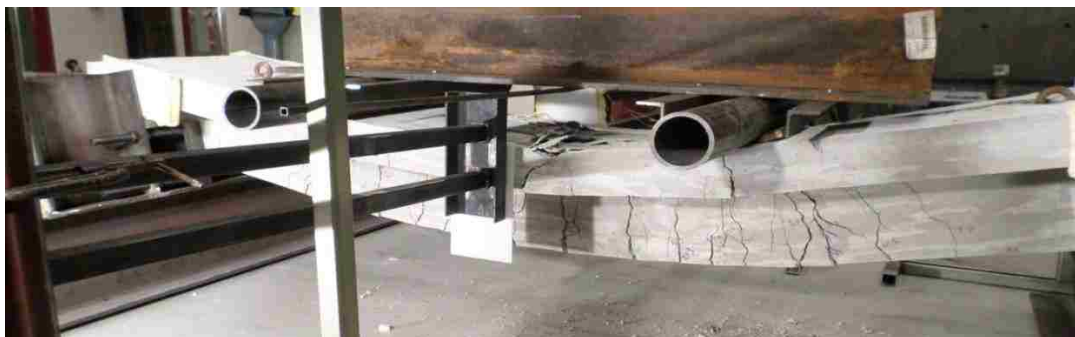
Figure 4.12: Beam-C at failure
