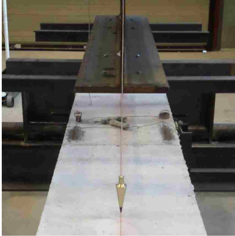
Figure 3.22: Beam centered under the loading beam showing also leveling device
