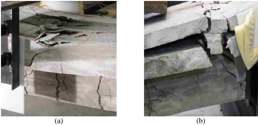
Figure 4.61: Failure mode for (a) Beam-C (b) Beam-UF
