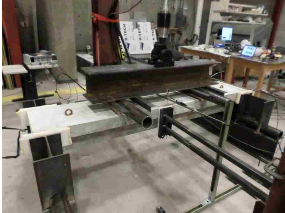
Figure 3.18: Four point bending setup for beams testing
