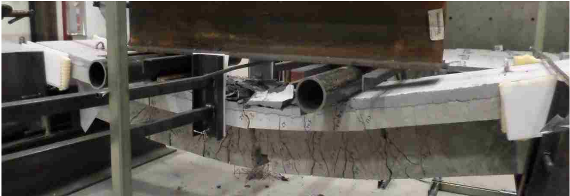
Figure 4.23: Beam-U at failure
