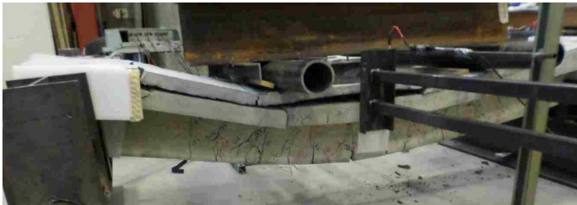
Figure 4.71: Debonding of LMUHPC overlay in Beam-MUF
