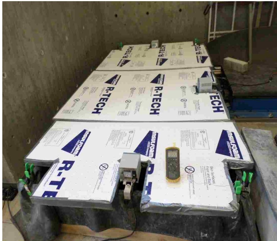
Figure 3.15: Curing tank used in the curing process
