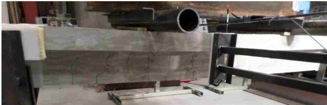
Figure 4.11: Cracks propagated in Beam-C
