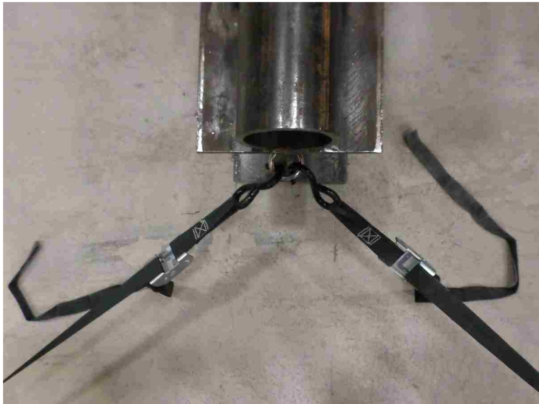
Figure 3.17: Support tie down
