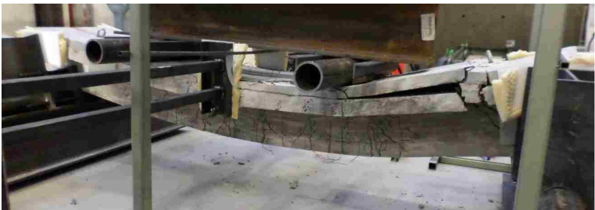
Figure 4.34: Beam-UF at failure
