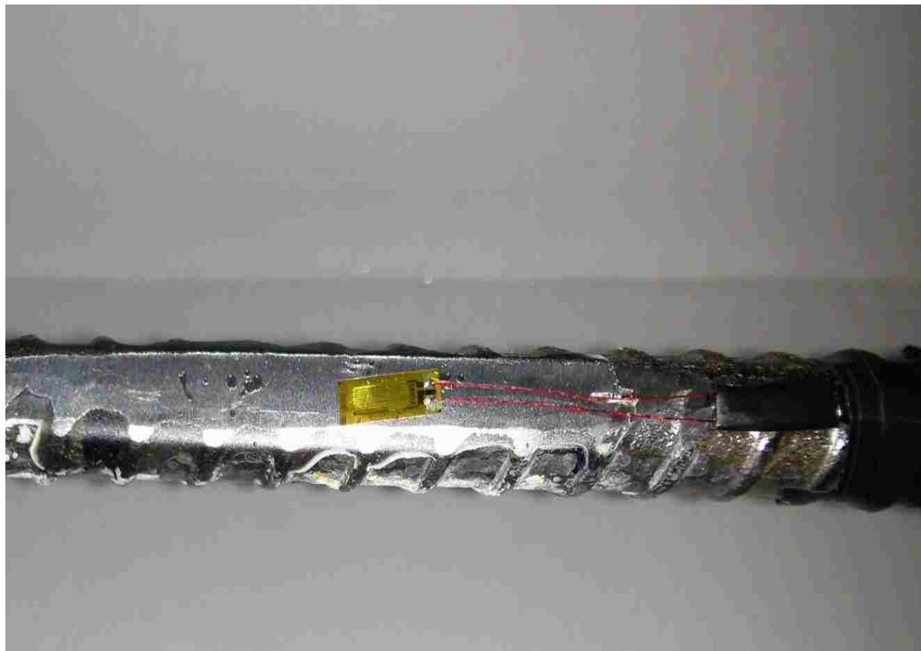
Figure 3.4: Strain gauge installed on steel rebar
