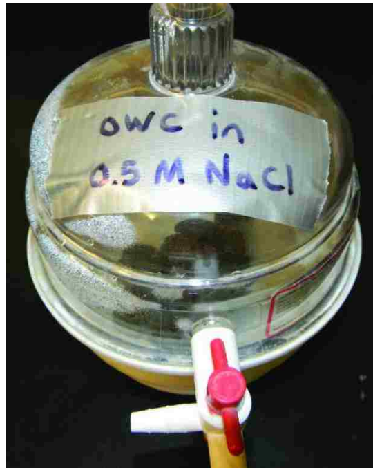
Figure 3.14 Degradation testing specimen conditioning setup
