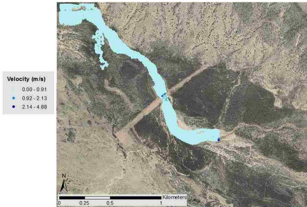
Figure 75: SRH-2D velocity results at 5.7 m 3 /s modeled discharge
