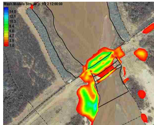
Figure 30: SRH-2D mesh – Hard steps no weir crest
