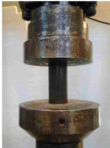
Figure 3.5: Compression test setup for cylinders.
