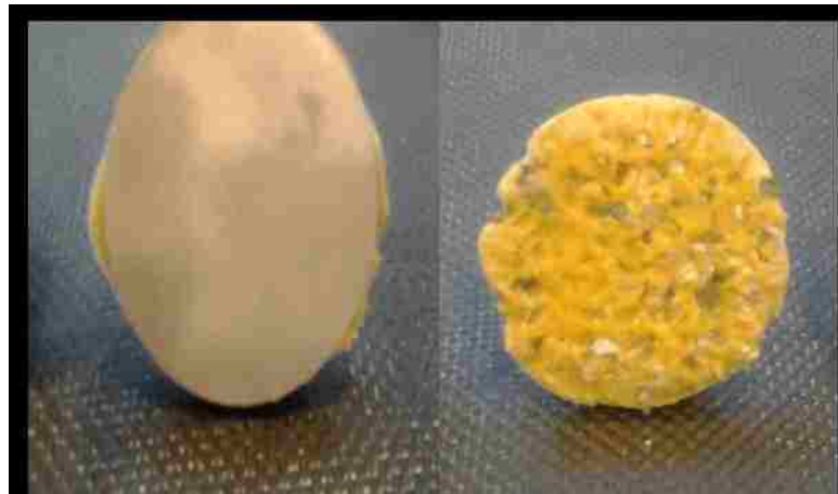
Figure 4.37: Second stage failure patterns, invalid pattern I on the left and valid result on the right (pattern III).
