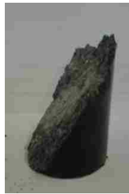
Figure 4.25: Cohesive shear failure under axial loading in the case of 1.5% MWCNTs.
