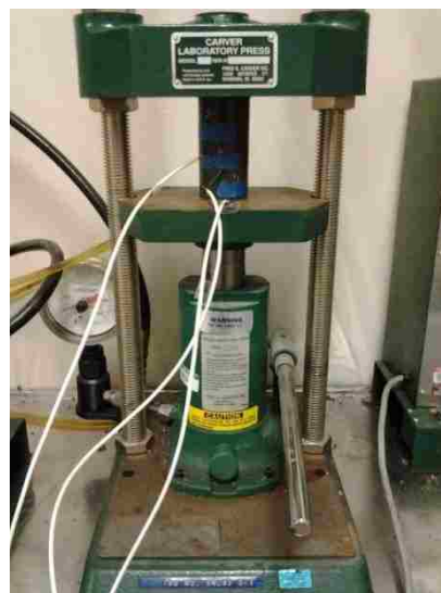
Figure 3.10: Creep test frame loaded with test specimen.
