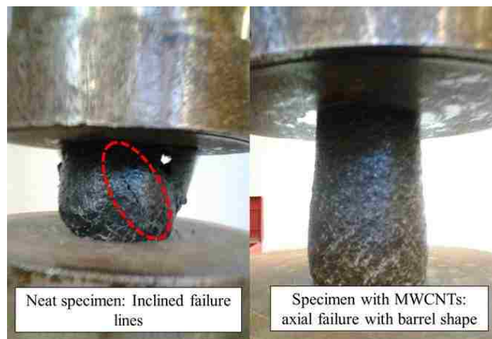
Figure 4.7: Different failure modes of Compressive strength test.
