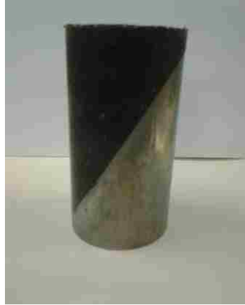
Figure 3.23: Composite cylinder test specimen of PC overlay on steel.
