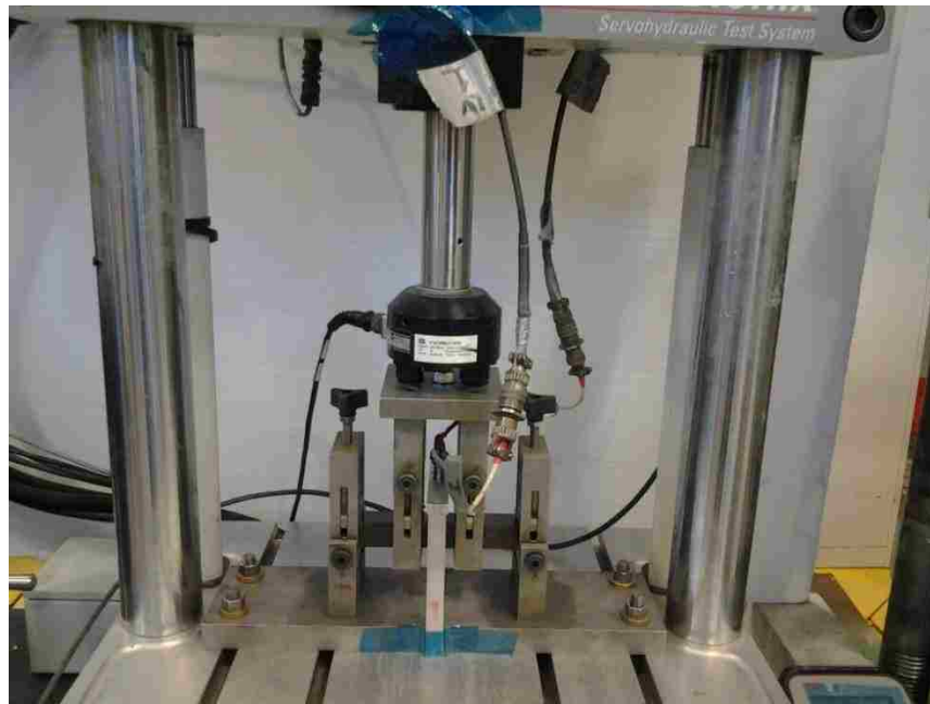
Figure 3.28: Four-point bending fatigue test setup.
