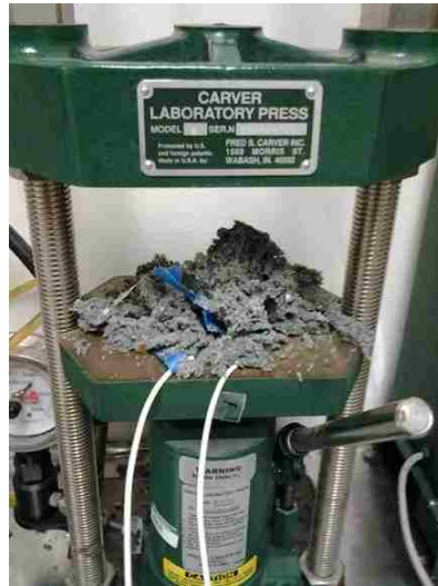
Figure 4.23: Crushing of PC specimens at failure under sustained axial loads.
