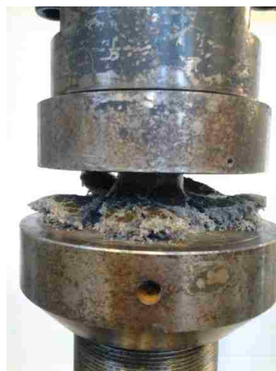
Figure 4.8: Crushing of PC specimens at failure under axial compression loads.
