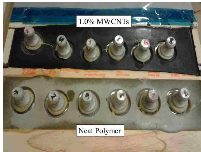
Figure 3.20: Fifth stage of pull off test setup.
