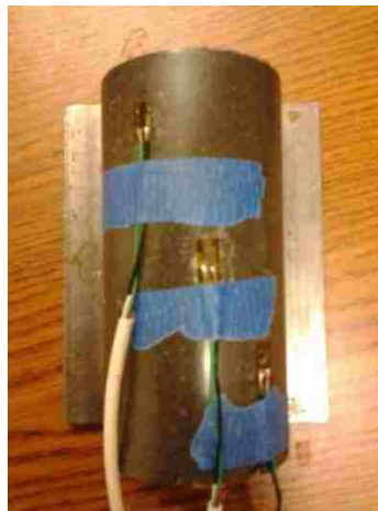
Figure 3.9: One creep test specimen with 3 strain gauges.
